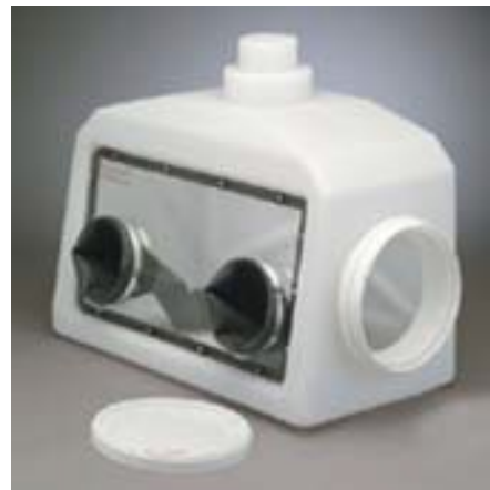
Glove box with venting capability
