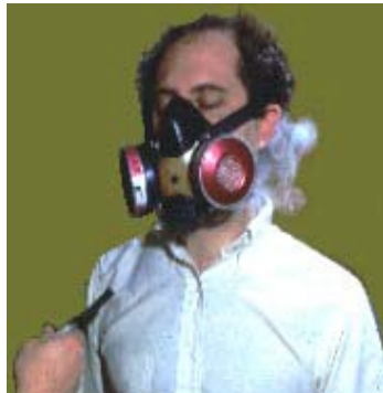
Fit testing a half mask with irritant smoke
