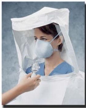
Fit testing an N-95 with Bitrex™
