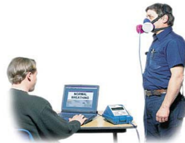
Fit testing a half mask using a Portacount™
