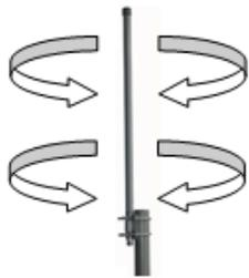
**Whip** - Antenna that radiates energy equally in all directions. Maintain as much distance as possible from this antenna.
