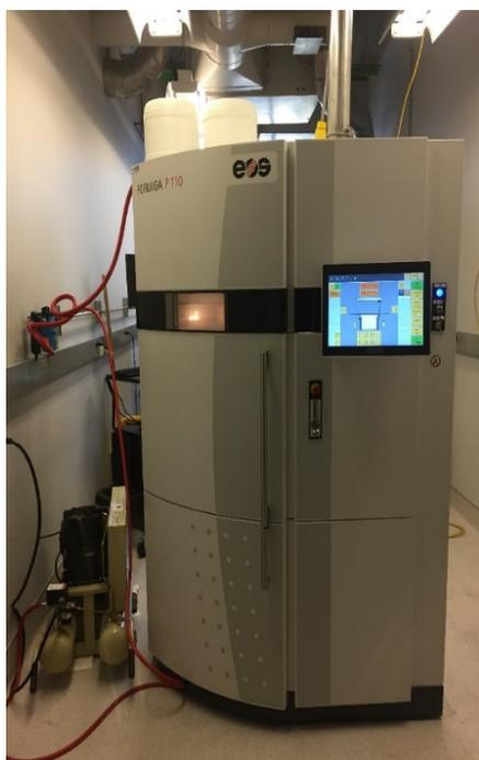
EOS Formiga P110 Laser Sintering 3D printer
